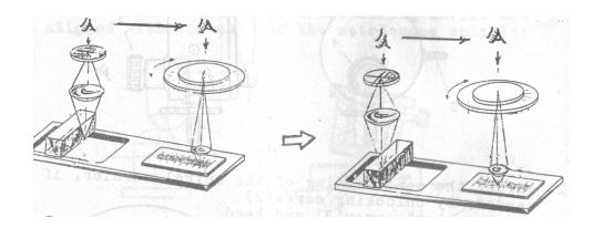
The Abbe comparator has a scale value of 0.001 mm and a measuring range of 200 mm with a maximum unreliability of  $\pm$  1.5  $\mu$ m over the total measuring range.
