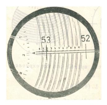
The image of the main scale millimeter graduations (scale marks 52 and 53), the eyepiece stationary linear scale having 10 graduations with a scale division of 0.01 mm (scale marks from 0 to 10), these scale marks being lined along the double radial line which end with an index; a section of the turning vernier circular scale graduated from 0 to 100 with a scale value of 0.001 mm; and a section of a double Archimedean spiral marked on the same gratitude as the circular scale.
