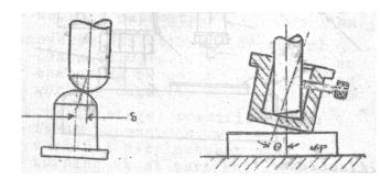
9. With Abbe horizontal comparator, be sure that the line of measurement is aligned to the measuring direction.
