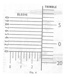
On the sleeve parallel to the datum line are graduated ten divisions which occupy the same space as nine divisions on the thimble. Thus one vernier division equals  $1/10 \times 9/1,000$  which is 9/10,000. The difference between a vernier and thimble division is 10/10,000 minus 9/10,000 which is 1/10,000 or  $0.0001^{\circ}$ .
