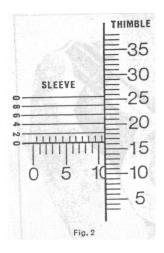
On the sleeve parallel to the datum line are graduated five divisions which occupy the same space as nine divisions on the thimble, each division on the vernier scale representing two thousandths of a millimeter (0.002 mm).
