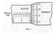
(N.B. On earlier models the millimeters are graduated above the datum line with half millimeters below).
