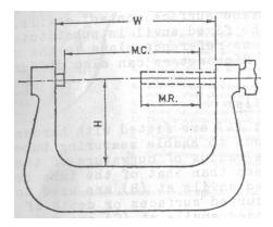
Standard U-frames are made according to the standard measuring capacities where the measuring range remains unchanged and equals to 25 mm.
